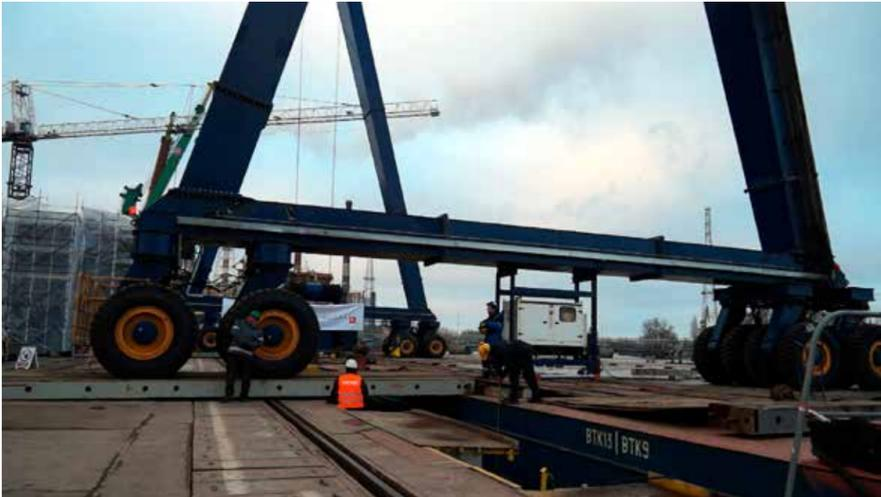
The new rubber wheeled gantry crane during rolling from a floating barge onto the shipyard's quay.
