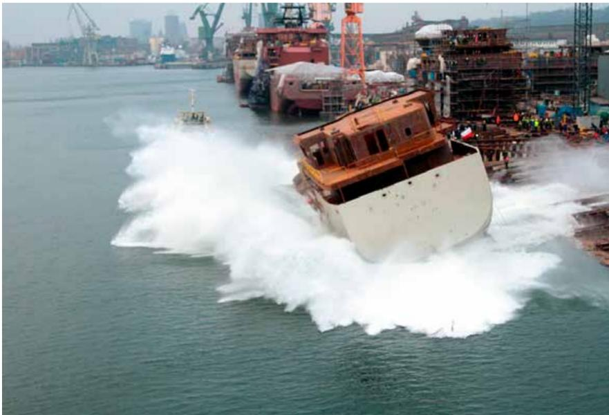
Side - launching of the 36 TEU arctic supply vessel at Remontowa Shipbuilding.
