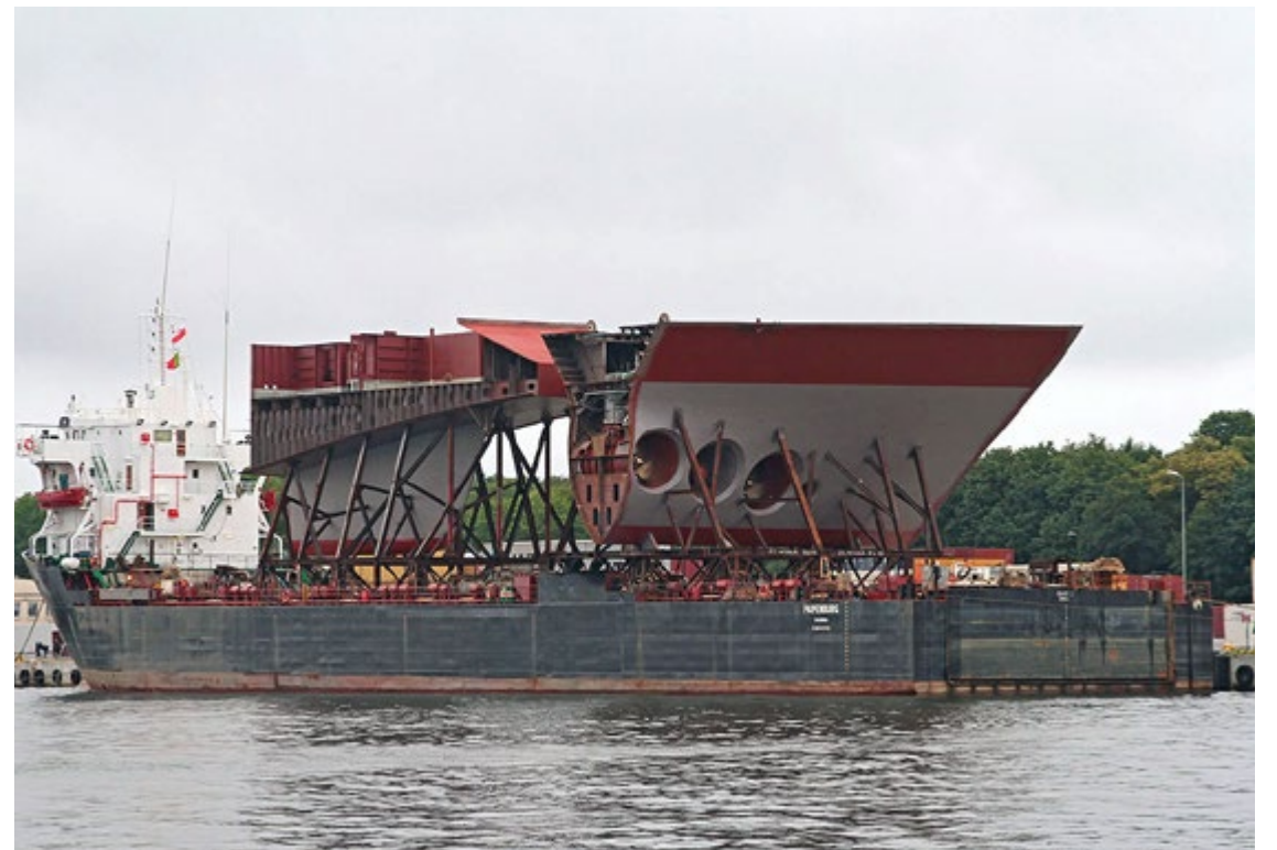
Earlier shipment (from Summer 2016) of ship sections for Norwegian Joy under construction at Meyer Werft.
