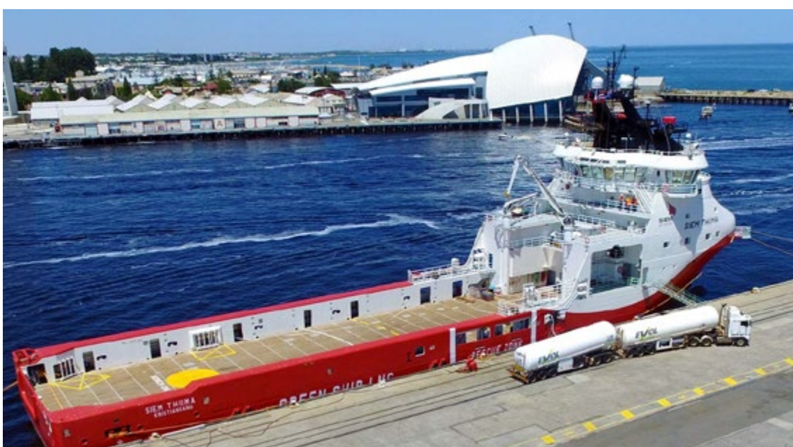
The Siem Thiima bunkering LNG at the King Bay Supply Base in Dampier, WA, January 23, 2017. Photo: EVOL LNG
