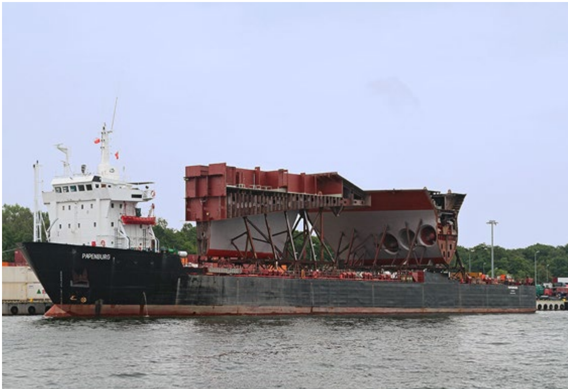
Earlier shipment (from Summer 2016) of ship sections for Norwegian Joy under construction at Meyer Werft.
