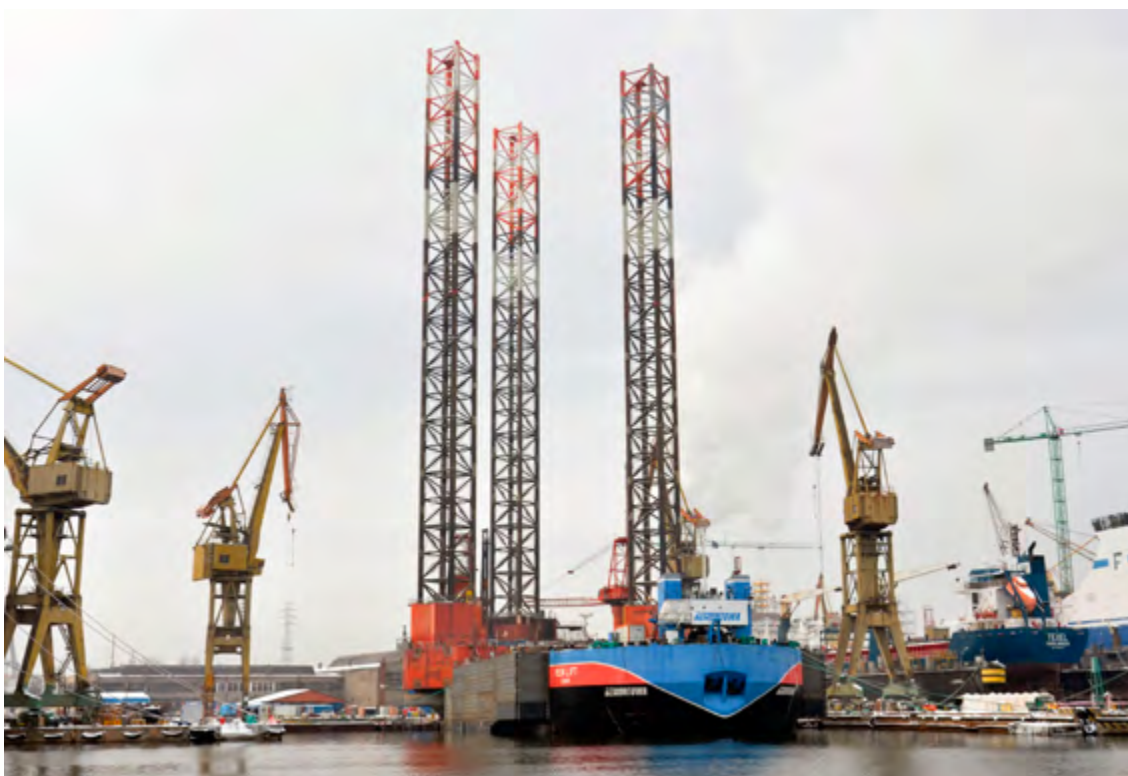
The Petrobaltic jack-up rig docked on board the REM Lift 25 000 submersible heavy lift unit at Remontowa SA.
