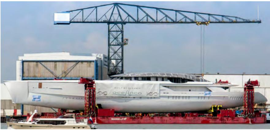
Sailing superyacht Y712 with superstructure from Aluship Technology on a launching pontoon-barge.
