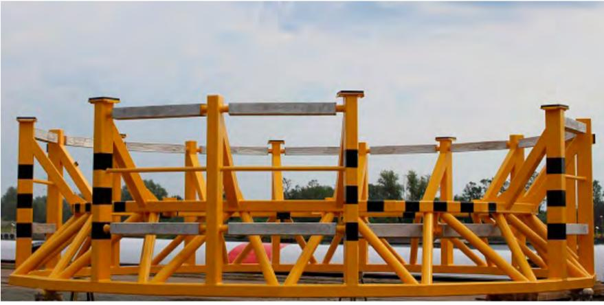
GSG fabricated anode cage.
