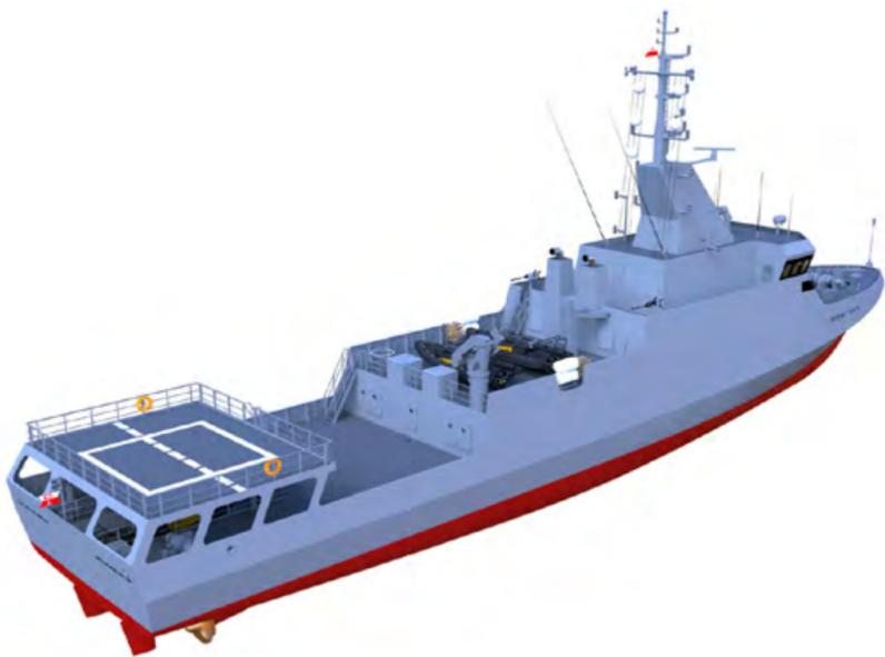
The primary task of the ship is to decrease or eliminate remnant magnetic field of other ships with a displacement of up to 6,000 ton, and measurements of physical fields (magnetic field, hydro-acoustic, electrical and thermal). Secondary tasks include search and rescue operations, towing operations and support for navy operations.
