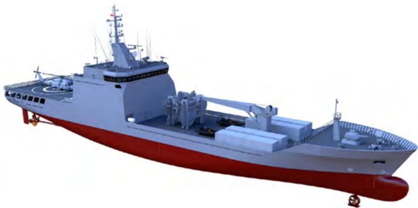
The main task of the ship is Replenishment at Sea (RAS) of Fuel and Water, and also other consumables to other surface operating Navy Vessels. Additional tasks will also include providing technical assistance for the repair and maintenance of military equipment. Principal particulars: length 106.0 m, breadth 18.0 m, design draft 5.0 m, speed (max) 20 kn, speed (service) 15 kn, displacement 5,700 t, capacity: fuel 1,800 m<sup>3</sup>, fresh water 200 m<sup>3</sup>.
