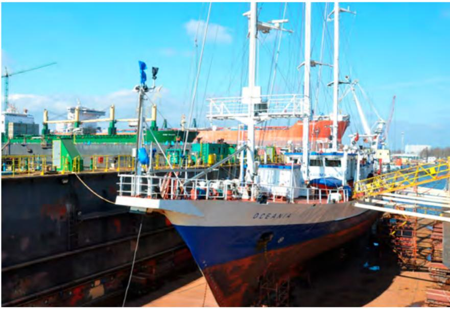
received a new lease of life, with modern outfitting of interiors and replaced - new or modernized ship's systems and functional equipment. At that occasion, even the whole engine room was upgraded with main engine replaced with new, twice as powerful unit as well as the bridge extended.
