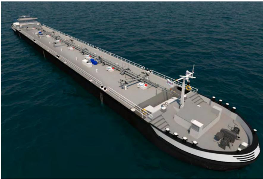
The new inland waterway barges with the hulls being built at Centromost shipyard, to be equipped with Wärtsilä dual-fuel engines and Wärtsilä LNGPac fuel gas handling systems.
