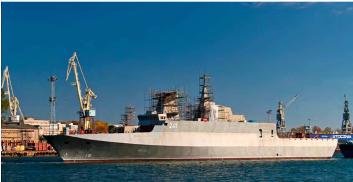
ORP Ślązak being towed just prior to lifting up on a syncrolift. Photo: Piotr B. Stareńczak
