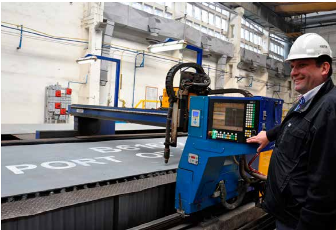
Allan Kiil starts the plasma cutting machine for steel plates. Photo: Ireneusz Gradkowski
