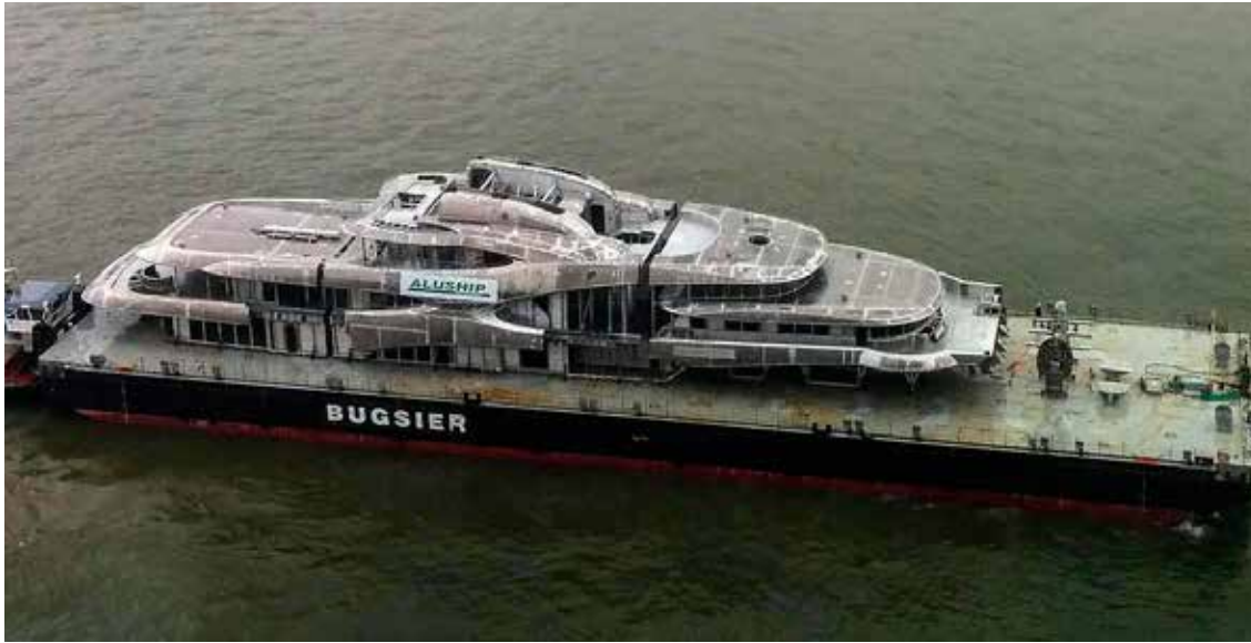
Superstructure from Aluship Technology on its way to the Netherlands. Photo: John Groenendijk
